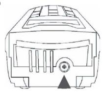
Select the correct antenna for the mobile radio system (extra accessory, see table on page 4) which matches the mobile phone frequency range and secure it to the TNC connection of your Willtek 4100 by tightening the coupling ring.
