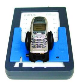
The important feature with the 4916 Antenna Coupler is that mobile phones of the same type can always be placed in the same position in the clamp.
